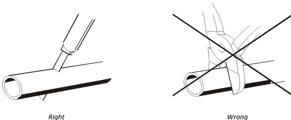
Fig. 8.8 Cutting the fuel line before installation
