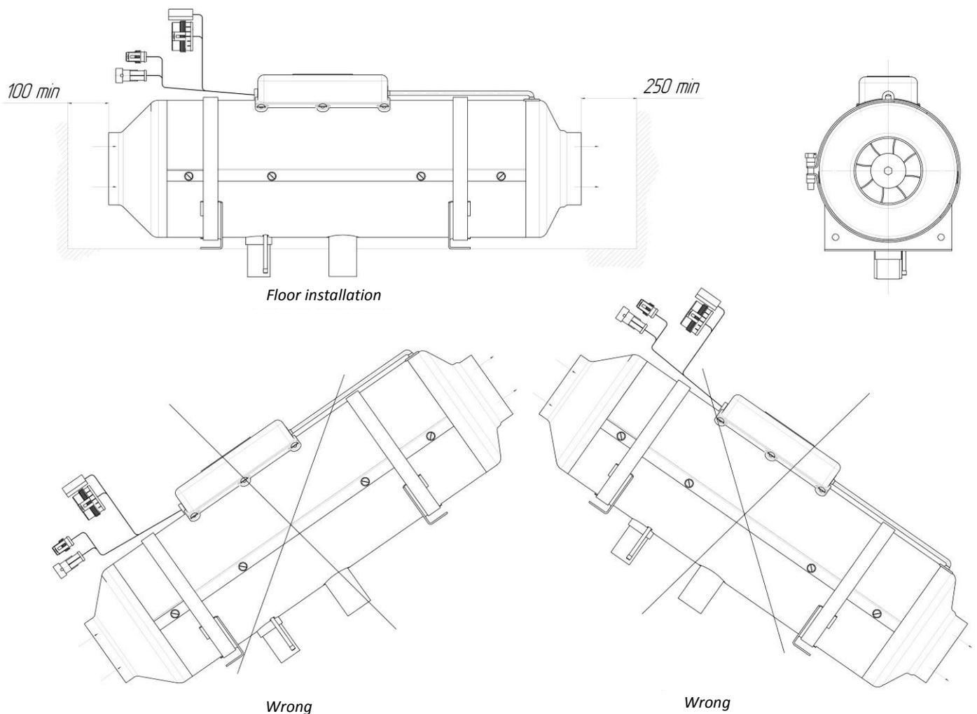
Fig. 8.1 Heater installation
