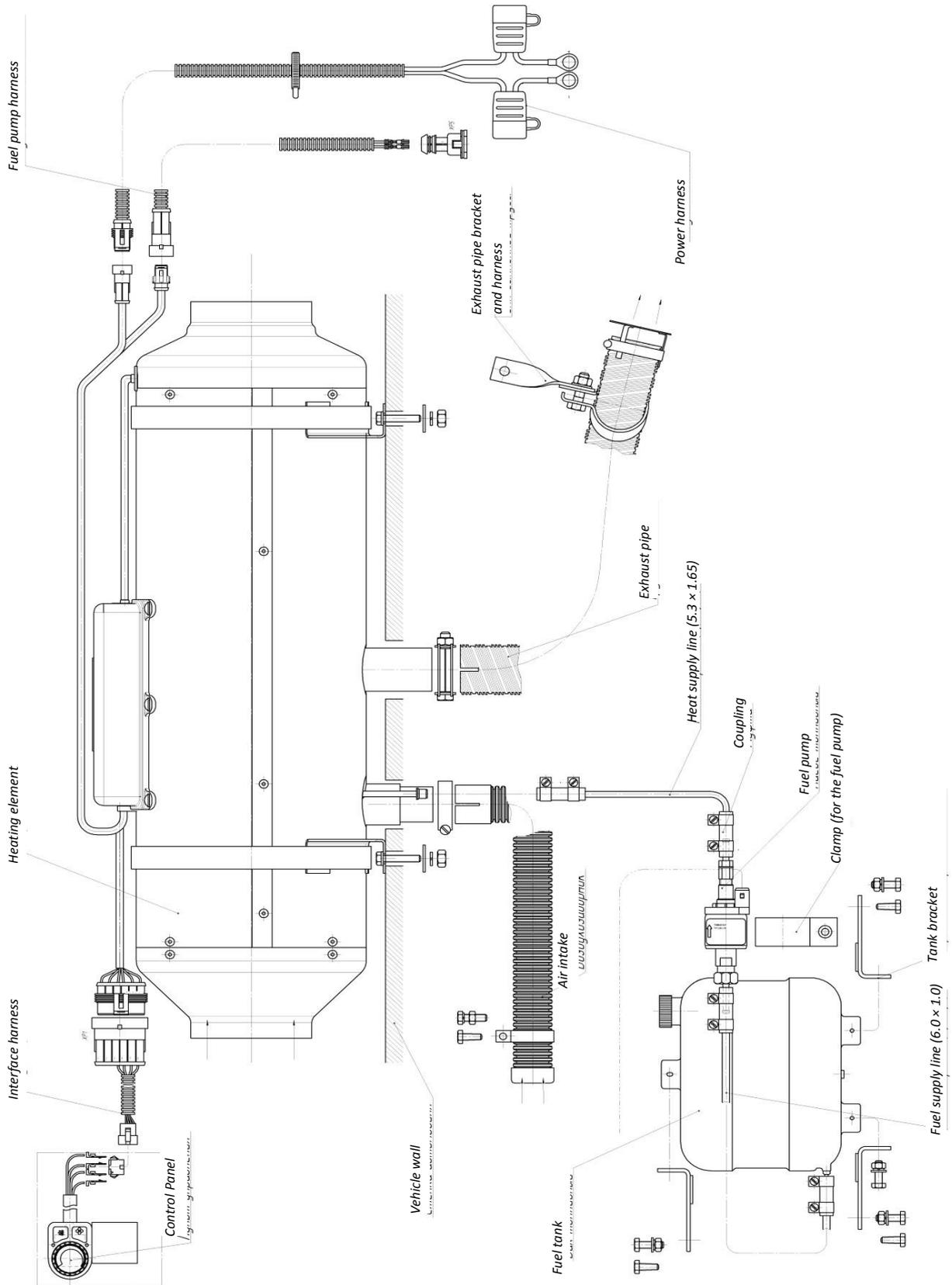
Fig. 7.1 Connections of main parts of the heater
