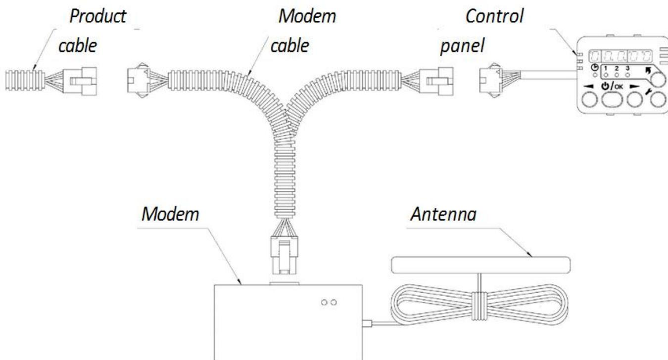
Fig.4 – Modem connections.
