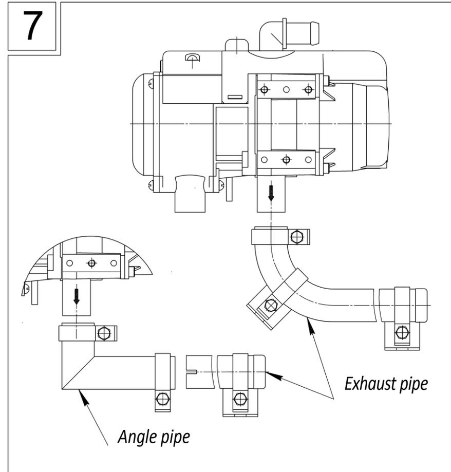
The exhaust pipe must be laid in a downward slanting direction from the pre-heater. If this not possible, then it is necessary to make a hole of size  $\text{Ø}3$  at the lowest point for discharge of condensate.
